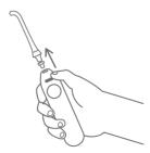
14 Press the Release Button on the handle, remove and dispose the irrigation tip.
