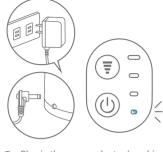
2 Plug in the power adapter (machine enters standby mode, light flashing).
